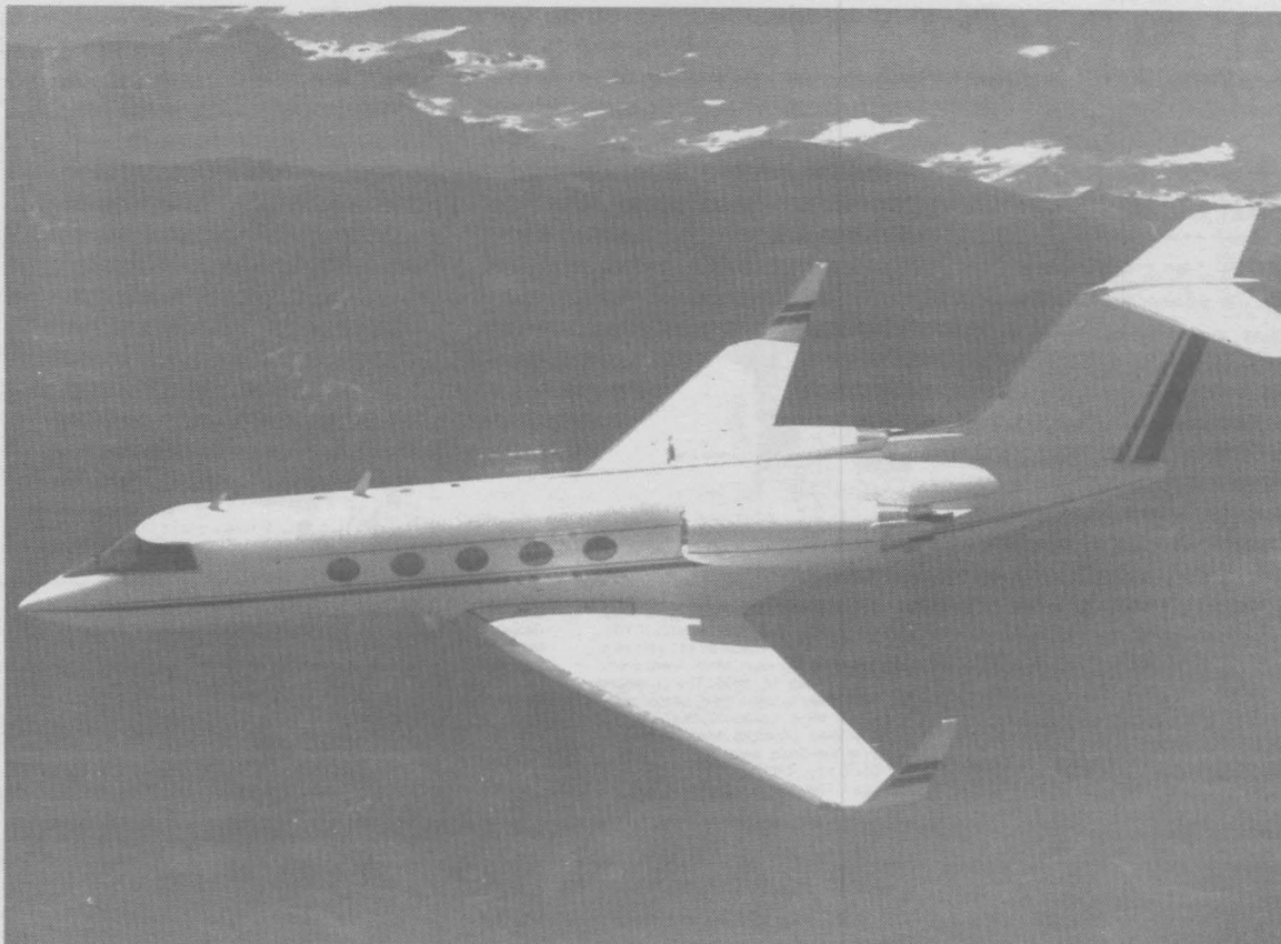
G-III IN FLIGHT — The G-III's winglets (the turned-up portion of the wing tips) cut wind drag by 3 percent, adding 133 miles to its flying range of 4,428 statute miles. [Photo by Warren Watson]
